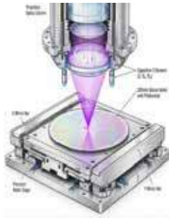
Fig. 1 Schematic diagram of a multi-DOF positioning sensor used in lithography wafer fabrication.
