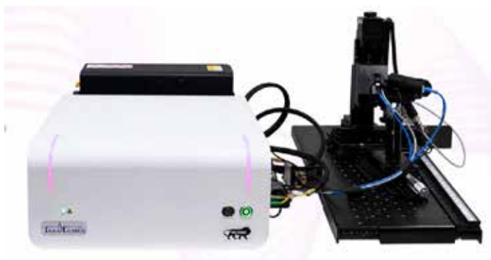
Fig. 3 Terahertz imaging system for cancer margin detection.
